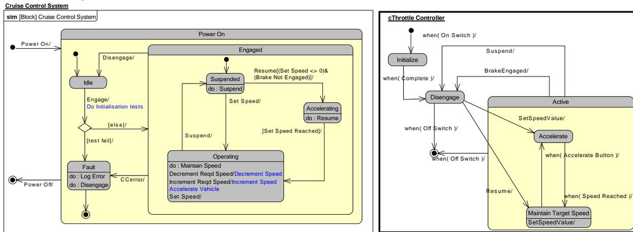
Figure 5. State diagrams for the Cruise Control System and Throttle Controller.
