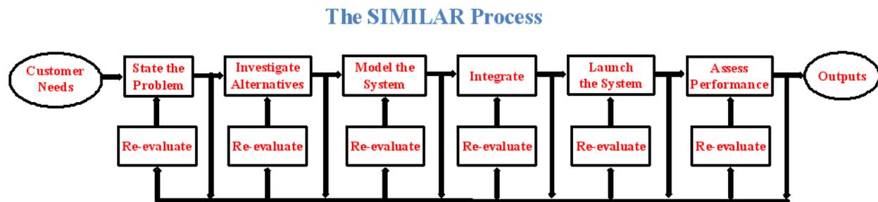
Figure 1. The Systems Engineering Process (Bahill, Gissing, 1998).
