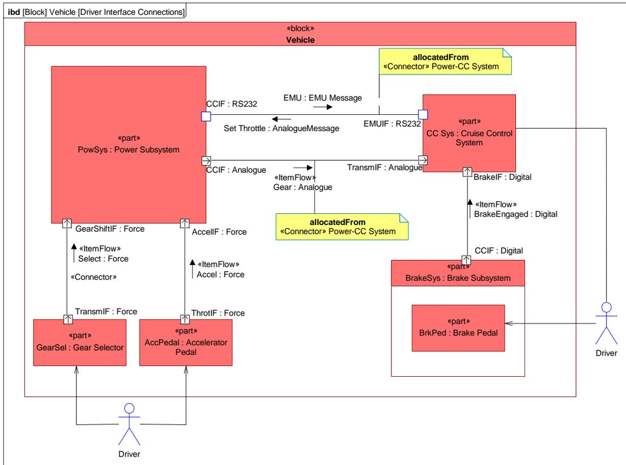
Figure 7. Cruise Control External Interfaces.
