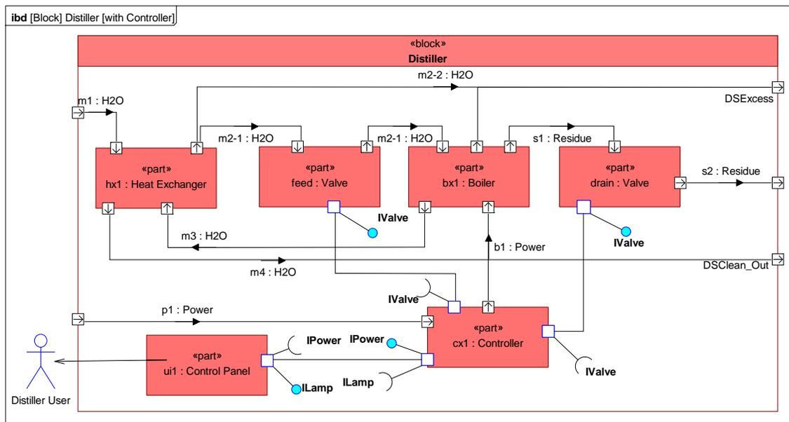
Figure 6. Distiller System With Controller.
