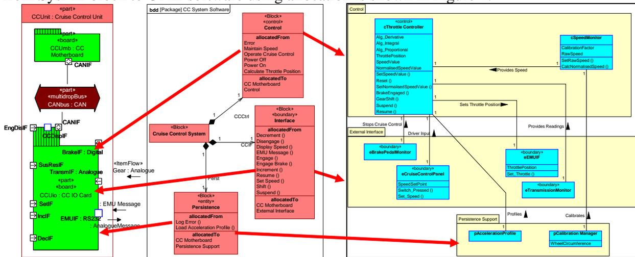
Figure 4. Mapping from Virtual Blocks to UML Packages and Hardware Platform.
