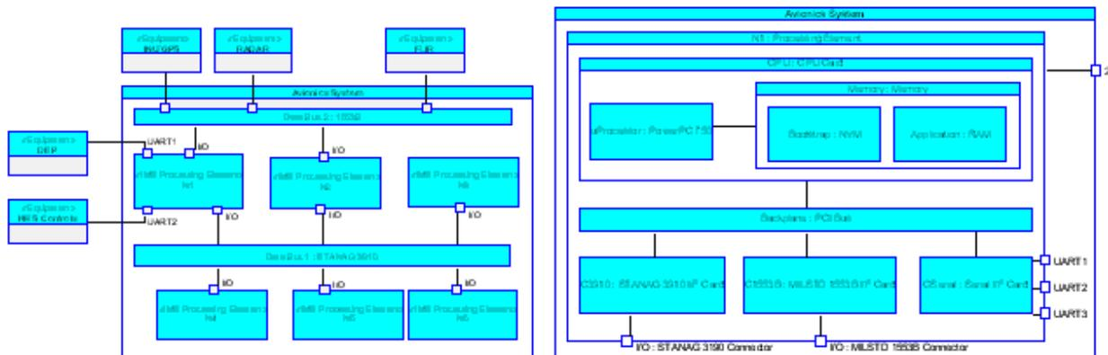
Figure 8. IMA Topology of Processing Elements and Internals of a Processing Element.
