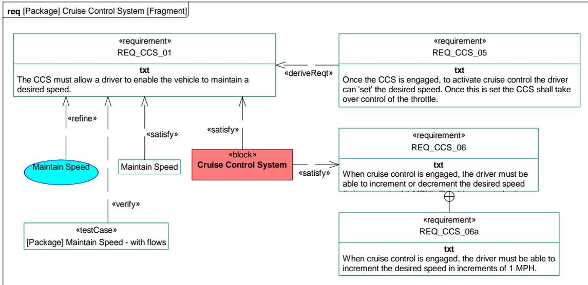
Figure 2. Requirements Example for a Cruise Control System
