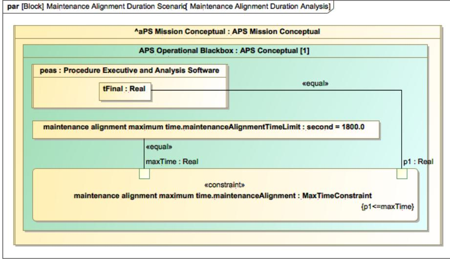
Figure 8. Connecting properties of APS to formalized requirements.
