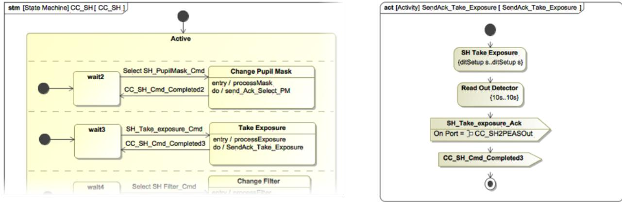
Figure 5. Specified behavior of SH filter (partial): (a) lifecycle behavior and (b) taking exposure.
