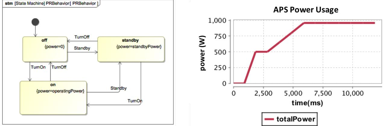
Figure 9. Peak power consumption analysis: (a) general pattern used and (b) result of executing analysis.
