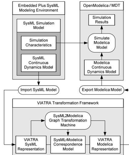
Figure 4. Functionality of the SysML-to-Modelica transformation Eclipse plug-in.
