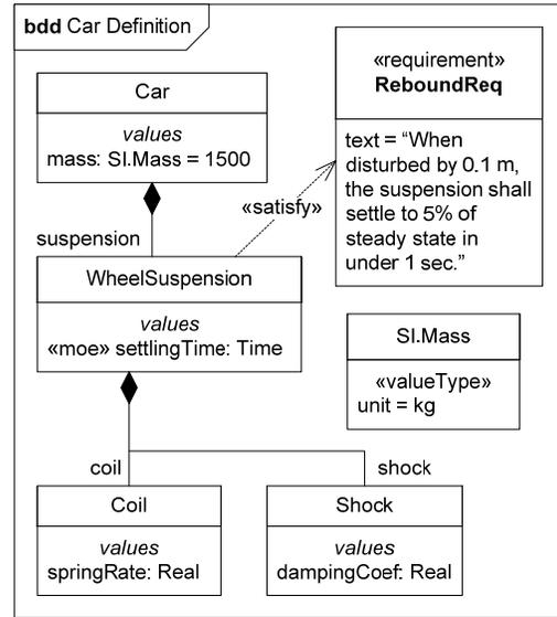
Figure 1. The SysML car suspension model.
