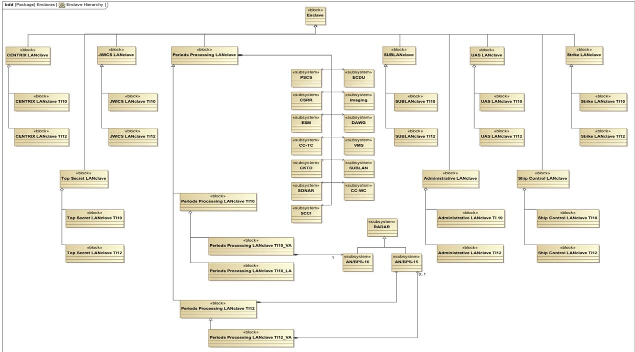
Fig. 6. CS2 Network Enclaves with Navigation Radar Assignments Migrating Across Network Enclaves with Evolving Baselines
