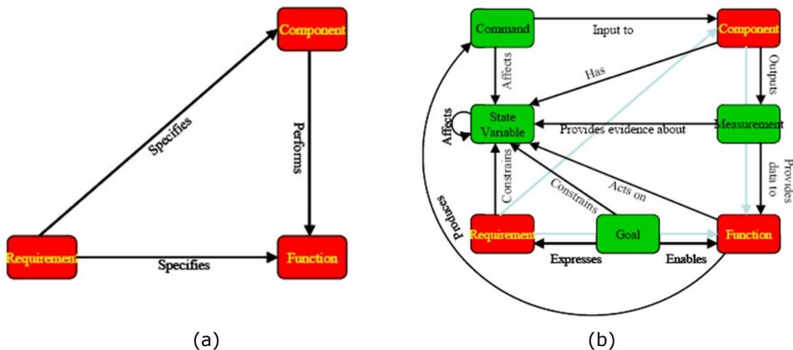
**Figure 3-20. (a) Functional Analysis Elements and Relationships, (b) Elements and Relationships of State Analysis Synthesized with Functional Analysis.<sup>12</sup>**
