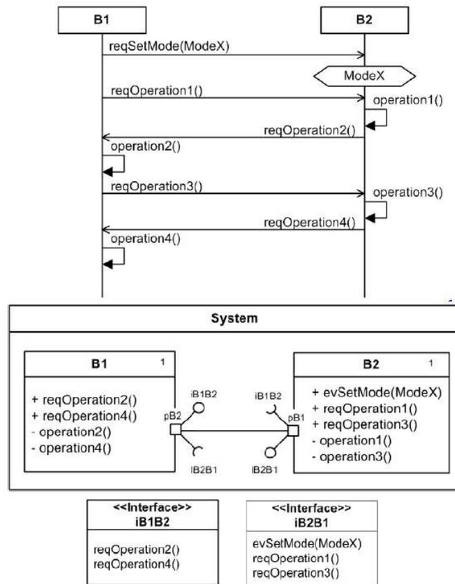
**Figure 3-2. OMG SysML™ Representation of Service Request-Driven Approach.**
