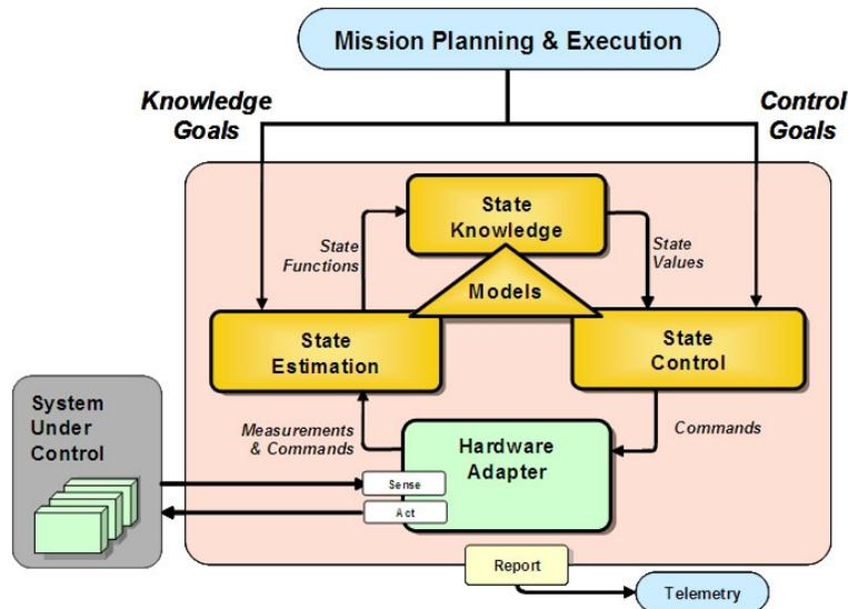
**Figure 3-18. Model- and State-Based Control Architecture ("Control Diamond").**
