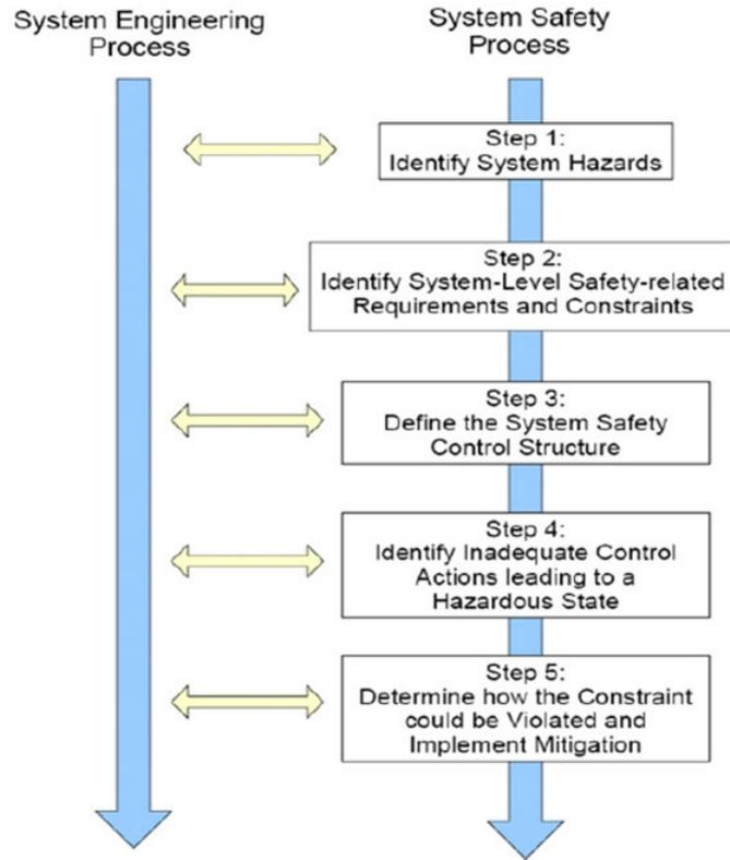
**Figure 3-21. Integrated Approach to Design for Safety.**
