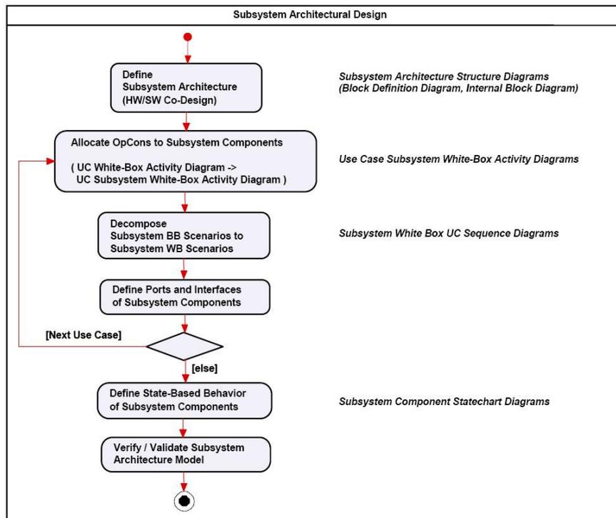
**Figure 3-5. Subsystem Architectural Design Task Flow and Work Products.**
