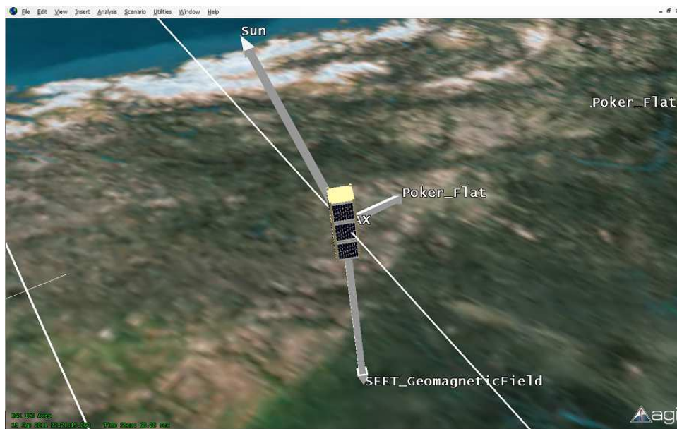
Figure 5. Schematic of RAX spacecraft with vectors pointing towards the experimental zone, Poker Flat, AK, the sun, and along the Earth's magnetic field (which the spacecraft long axis is aligned with). The figure is generated using STK.
