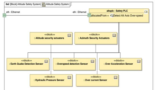
Figure 9 Allocation of behavior to structure
