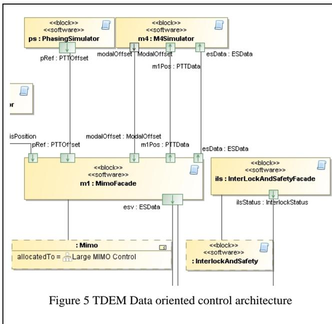
Figure 5 TDEM Data oriented control architecture
