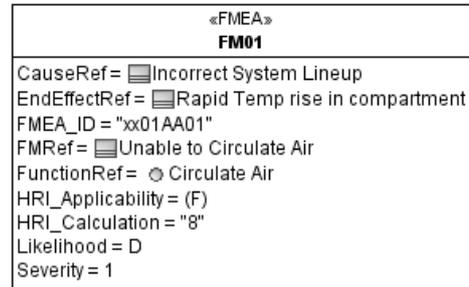
Figure 17. Example FMEA for an HVAC System
