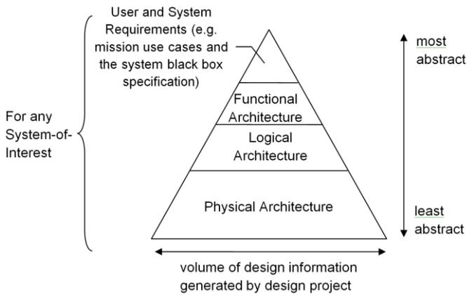
Figure 3. Levels of System Architecture and Abstraction
