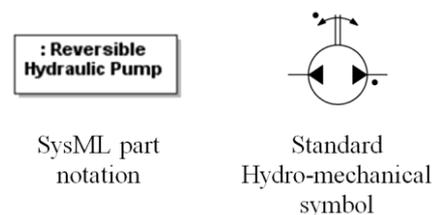
Figure 14. Comparing SysML part notation with an industry-standard hydromechanical symbol
