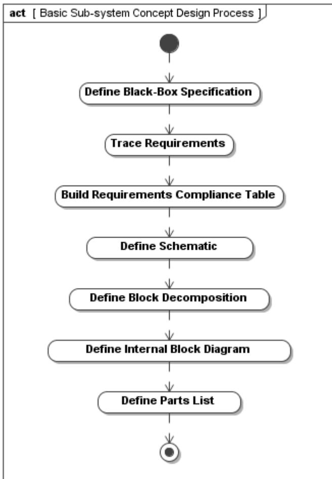
Figure 8. Basic Subsystem Concept Design Process
