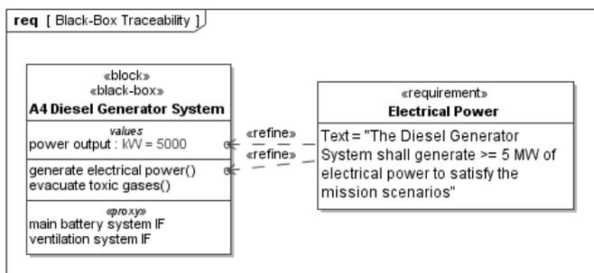
Figure 2. Example Black-Box Specification in SysML
