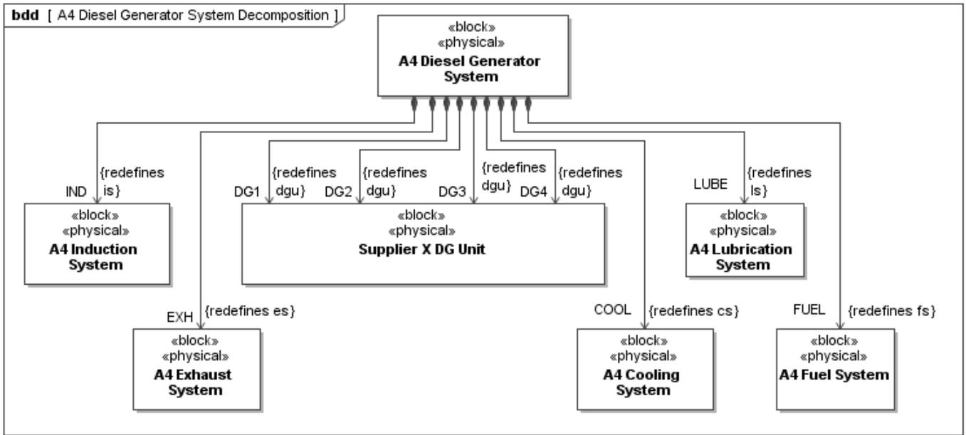
Figure 12. Subsystem Block Decomposition Diagram
