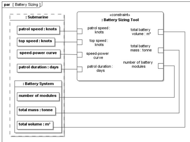
Figure 19. SysML Parametric Example: Battery Sizing Tool
