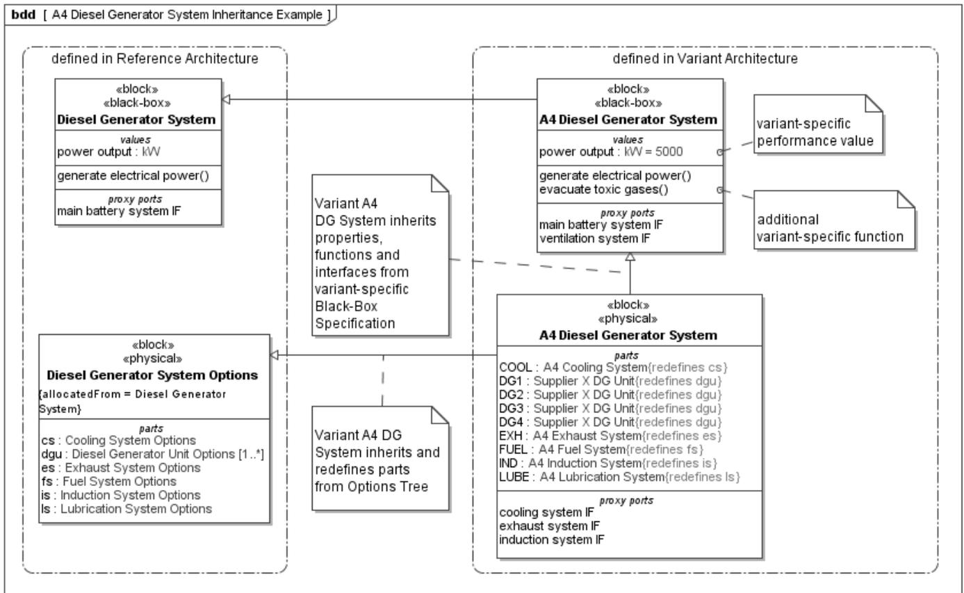
Figure 7. Example: Building a Physical Variant Design using Inheritance
